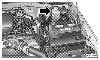
Be sure to clean the top of the master cylinder area before removing the cap. If necessary, add fluid to bring the fluid level up to the requirements described on the brake fluid reservoir. With disc brakes, fluid level can be expected to fall as the brake pads wear. However, low fluid level may be caused by a leak and a checkup may be needed.
