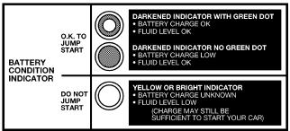
To determine the battery charge, check the battery test indicator (if equipped) on top of the battery. Refer to the illustration.
