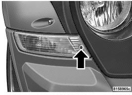
2. Pull the inboard side of the lamp away enough to disengage the tab that secures the outboard side of the lamp from the slot in the front bumper fascia.
