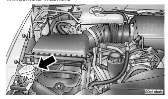
The fluid reservoir for the windshield washers and the rear window washer is shared. It is located in the front of the engine compartment on the passenger side and should be checked for fluid level at regular intervals. Fill the reservoir with windshield washer solvent (not antifreeze/coolant) and operate the system for a few seconds to flush out the residual water.
