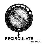
Use this button to choose between outside air intake or recirculation of the air inside the vehicle. A lamp will illuminate when you are in recirculate mode. Only use the recirculate mode to temporarily block out any outside odors, smoke, or dust and to cool the interior rapidly upon initial
