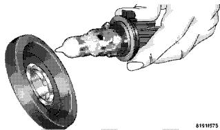
Removing Halogen Bulb From Assembly
