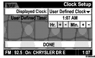
2. To increase the clock by hours, make sure "HR +" is highlighted and press ENTER. Press ENTER again to increase the clock by another hour. You will see on the "User Defined Time" display the number of hours you have increased the clock by.
