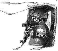
Removing Socket and Bulb
