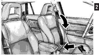
Inserting Latch Plate Into Buckle
