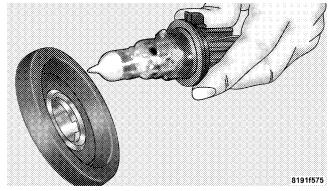
**Removing Halogen Bulb From Assembly**
