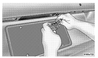
**Removing Socket from Lamp**
