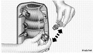
**Removing Bulb From Socket**
