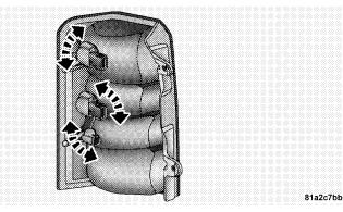
**Removing Socket and Bulb**
