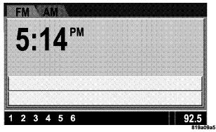
3. To switch the clock to the small clock, quickly press TIME again.
