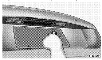
**Prying Lamp from Liftgate** 2. Rotate the socket 1/4 turn counterclockwise.
