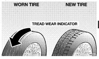
These indicators are molded into the bottom of the tread grooves. They will appear as bands when the tread depth becomes 1/16 inch (2 mm). When the tread is worn to the tread wear indicators, the tire should be replaced.
