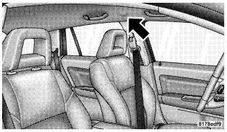
Side Curtain Airbag Location NOTE: Airbag covers may not be obvious in the interior trim; but they will open to allow airbag deployment.
