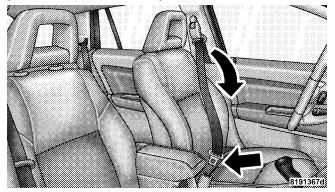
**Inserting Latch Plate Into Buckle**
