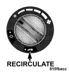
Use this button to choose between outside air intake or recirculation of the air inside the vehicle. A lamp will illuminate when you are in recirculate mode. Only use the recirculate mode to temporarily **4** block out any outside odors, smoke, or dust and to cool the interior rapidly upon initial
