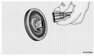
Remove green connector from back of bulb by pulling straight back
