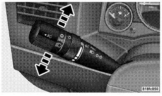
**Turn Signal Control** Move the Multi-Function Control Lever up or down and the arrows on each side of the instrument cluster flash to
