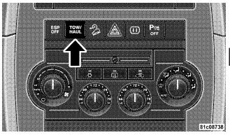
TOW/HAUL Switch The "TOW/HAUL" light will illuminate in the instrument cluster to indicate when the switch has been
