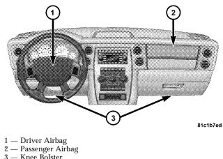
This vehicle has airbags for both the driver and right front passenger as a supplement to the seat belt restraint systems. The driver's front airbag is mounted in the steering wheel. The passenger side airbag is mounted in the instrument panel, above the glove compartment. The words SRS/AIRBAG are embossed on the airbag covers.
