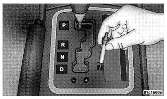
5. Move the shift lever into the N (Neutral) position.
