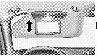
**Lighted Vanity Mirror** Sun Visor Extension (If Equipped) This feature has a pull out extension on the sun visor for increased coverage.
