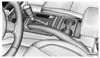
**NOTE:** The cup holder insert is removable, from the console, for cleaning. It can be reinstalled with the larger cup depression towards the passenger seat, but the top surface will not be flush with the console surface.
