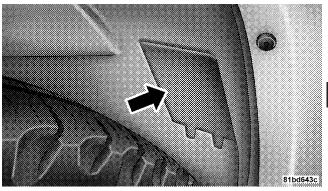
3. Reach through the access hole to access the back of the front fog light housing on the back of the front fascia.
