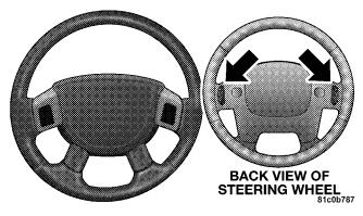
The right hand control is a rocker type switch with a push-button in the center and controls the volume and mode of the sound system. Pressing the top of the rocker switch will increase the volume and pressing the bottom of the rocker switch will decrease the volume.
