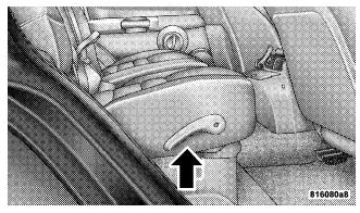
**Seatback Release Lever** 2. Fold the seatback down, and tumble the seat forward.
