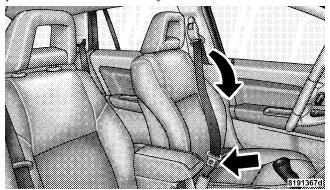
**Inserting Latch Plate Into Buckle**
