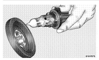
Removing Halogen Bulb From Assembly
