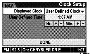
2. To increase the clock by hours, make sure "HR +" is highlighted and press ENTER. Press ENTER again to increase the clock by another hour. You will see on the "User Defined Time" display the number of hours you have increased the clock by.
