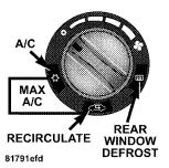
For maximum cooling use the A/C and recirculate buttons at the same time.
