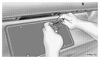
**Removing Socket from Lamp**
