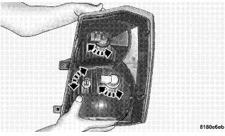
**Removing Socket and Bulb**
