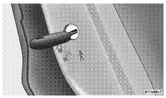
**Inserting Ignition Key**
