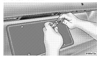
**Removing Bulb From Socket**
