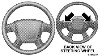
The right hand control is a rocker type switch with a push button in the center. Pressing the top of the switch will increase the volume and pressing the bottom of the switch will decrease the volume.
