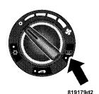
The push-button is located on the bottom right side of the blower control knob. Press. this button to turn on the rear window defroster. An amber light shows that the defroster is on.
