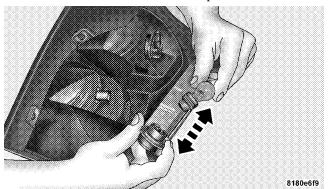
**Removing Bulb From Socket**
