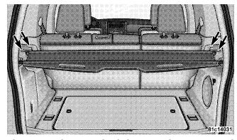
Then, insert the spring-loaded post on the opposite end of the cover housing into the attachment point on the opposite side of the vehicle.
