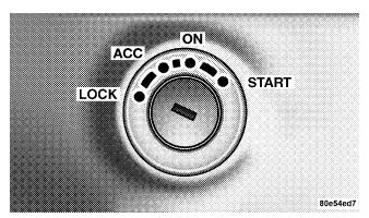
**Ignition Key Positions** Manual Transmission — If Equipped
