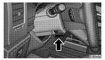
To unlock the steering column, push the control handle downward. To tilt the steering column, move the steering wheel upward or downward as desired. To lock the steering column in position, pull the control handle upward until fully engaged.
