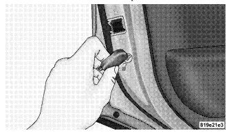
**Inserting Ignition Key**
