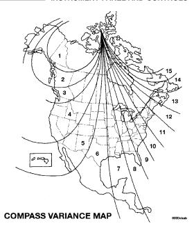
**NOTE:** The factory default zone is 8. During programming, the zone value will wrap around from zone 15 to zone 1.
