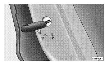
**Inserting Ignition Key**
