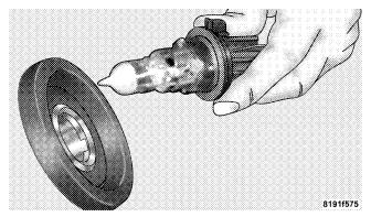
Removing Halogen Bulb From Assembly
