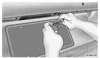
Removing Socket From Lamp
