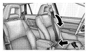
**Inserting Latch Plate Into Buckle**
