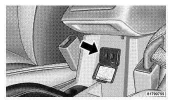
Power Outlet — 115 Volts (150 Watts)
