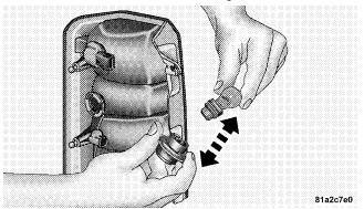
Removing Bulb From Socket
