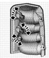
Removing Socket and Bulb
