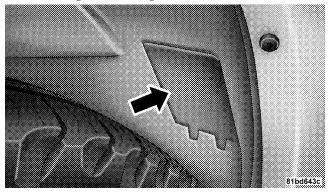
3. Reach through the access hole to access the park/turn signal bulb socket on the bottom of the front lamp unit housing.
