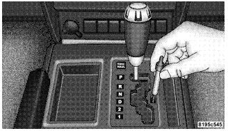
Shift Lock Manual Override6. Move the shift lever into the NEUTRAL position.
