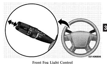
**NOTE:** The front fog lights will only operate with the headlights on low beam. Selecting high beam headlights will turn off the front fog lights.
