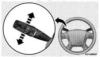
You can signal a lane change by moving the multifunction lever upward or downward partially without moving beyond the detent.
