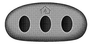
HomeLink<sup>®</sup> Buttons NOTE: HomeLink<sup>®</sup> is disabled when the Vehicle Security Alarm is active.
