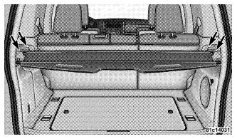
**Installing Retractable Cargo Area Cover** Then, insert the spring-loaded post on the opposite end of the cover housing into the attachment point on the opposite side of the vehicle.
