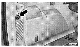
Cargo Tie-Down Loops Cargo tie-down loops are located on the trim panels.
