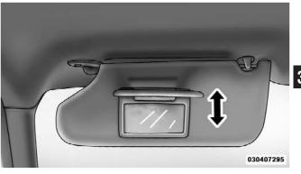
Illuminated Vanity Mirror Sun Visor "Slide-On Rod" Feature — If Equipped The sun visor "Slide-On Rod" feature allows for additional flexibility in positioning the visor to block out the sun.
