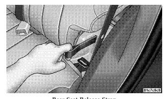
**Rear Seat Release Strap** 3. Fold the rear seat completely forward.
