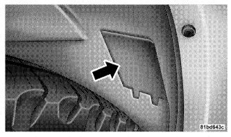
3. Reach through the access hole to access the park/turn signal bulb socket on the bottom of the front lamp unit housing.
