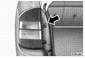
2. Grasp the taillamp and pull firmly to disengage the lamp from the aperture panel.
