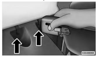
Using the handle, pull the cover toward you and guide the rear cover posts into the guides located on both sides of the rear trim panel.
