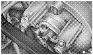
2. Reach into the engine compartment and pull the red lock out at the green connector.
