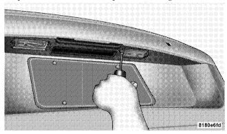
2. Rotate the socket 1/4 turn counterclockwise.
