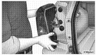
3. Twist and remove socket from lamp.
