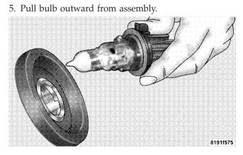
**NOTE:** These are halogen bulbs. Take care not to touch the bulb with your fingers. Body oils from your fingers could cause excessive heat buildup which reduces bulb life.
