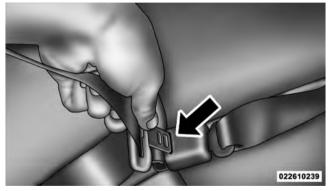
**Detaching Mini-Latch And Buckle** 10. To disengage the mini-latch from the mini-buckle for storage, insert the regular latch plate into the black
