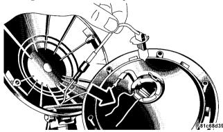
2. Unlatch the wire clasp securing the bulb into the 3. Disconnect the bulb from the lamp harness to replace the bulb.
