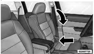
**Inserting Latch Plate Into Buckle**
