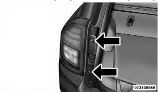
2. Grasp the taillamp and pull firmly to disengage the lamp from the aperture panel.
