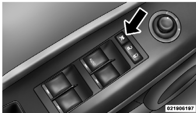
Window Lockout Switch
