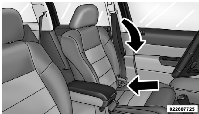
Inserting Latch Plate Into Buckle
