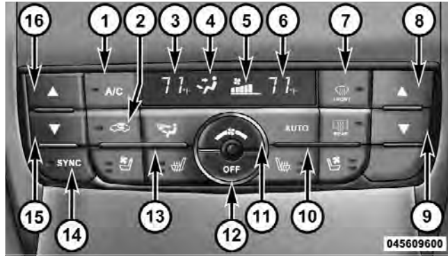
Automatic Temperature Control (ATC) Panel
