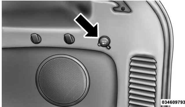
Rear Power Outlet
