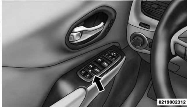
Window Lockout Switch
