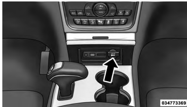
Front Power Outlet
