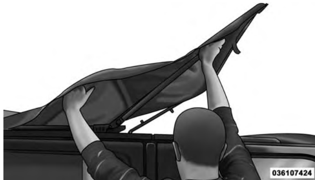
4. Engage the header latches.
