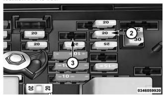
Rear Cargo Electrical Power Outlet Fuse
