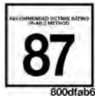
These engines are designed to meet all emissions regulations and provide excellent fuel economy and performance when using high quality unleaded "regular" gasoline having an octane rating of 87. The use of premium gasoline is not recommended, as it will not provide any benefit over regular gasoline in these engines.
