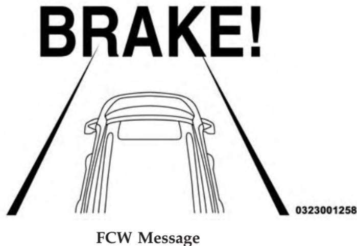
When the system determines a collision with the vehicle in front of you is no longer probable, the warning message will be deactivated.
