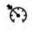
Turn the Normal (Fixed Speed) Electronic Speed Control ON. When the vehicle has reached the desired speed, push the SET (+) or SET (-) button and release. Release the accelerator and the vehicle will operate at the selected speed.
