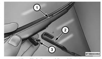
Wiper Blade Removed From Wiper Arm
