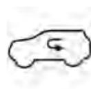
When outside air contains smoke, odors, or high humidity, or if rapid cooling is desired, you may wish to recirculate interior air by pressing the Recirculation control button. The recirculation indicator will illuminate when this button is selected. Press the button a second time to turn off the Recirculation mode and allow outside air into the vehicle.
