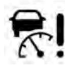
This light will illuminate when an ACC is not operating and needs service. For further information, refer to “Adaptive Cruise Control (ACC)” in “Understanding The Features Of Your Vehicle.”
