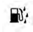
The “Water In Fuel Indicator Light” will illuminate when there is water detected in the fuel filters. If this light remains on, DO NOT start the vehicle before you drain the water from the fuel filters to prevent engine damage. Refer to “Maintenance Procedures/Draining Fuel/Water Separator Filters” in “Maintaining Your Vehicle” for further information.
