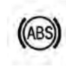
This light monitors the Anti-Lock Brake System (ABS). The light will turn on when the ignition switch is turned to the ON/RUN position and may stay on for as long as four seconds.
