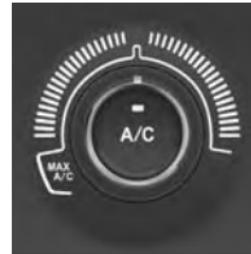
Use this control to regulate the temperature of the air inside the passenger compartment. Rotating the knob counterclockwise, from top center into the blue area of the scale, indicates cooler temperatures. Rotating the knob clockwise, into the red area, indicates warmer temperatures.
