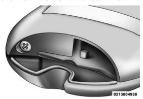
Remove Screw From Transmitter Case
