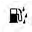
The “Water In Fuel Indicator Light” will illuminate when there is water detected in the fuel filters. If this light remains illuminated, DO NOT start the vehicle before you drain the water from the fuel filters to prevent engine damage. Refer to “Maintenance Procedures/Draining Fuel/Water Separator Filters” in “Maintaining Your Vehicle” for further information.
