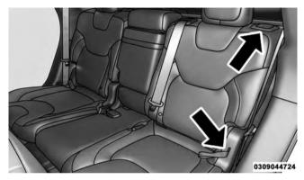
Rear Seatback Release Lever And Pull Strap
