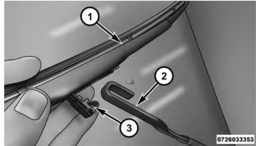
Wiper Blade Removed From Wiper Arm
