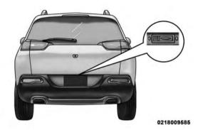
Electronic Liftgate Release/Liftgate Passive Entry Location
