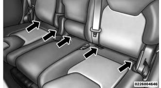
Rear Seat LATCH Anchorages Locating Tether Anchorages
