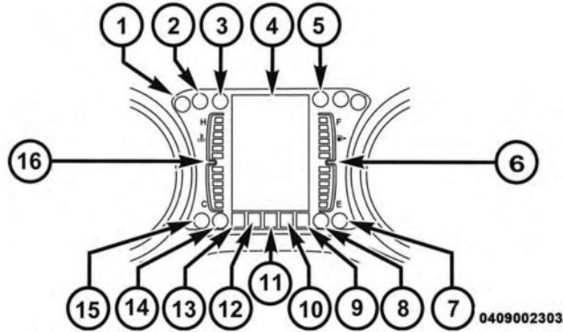
1. Electronic Park Brake Failure — If Equipped
