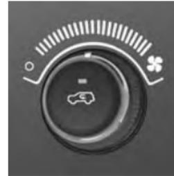
There are several blower speeds. Use this control to regulate the amount of air forced through the system in any mode you select. The blower speed increases as you move the control clockwise from the OFF position.
