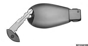
Separating Ignition Node Module (IGNM) Transmitter
