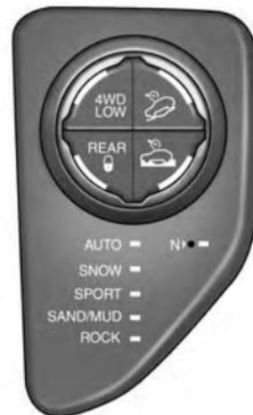
2-Speed 4x4 Switch (with Rear Lock)
