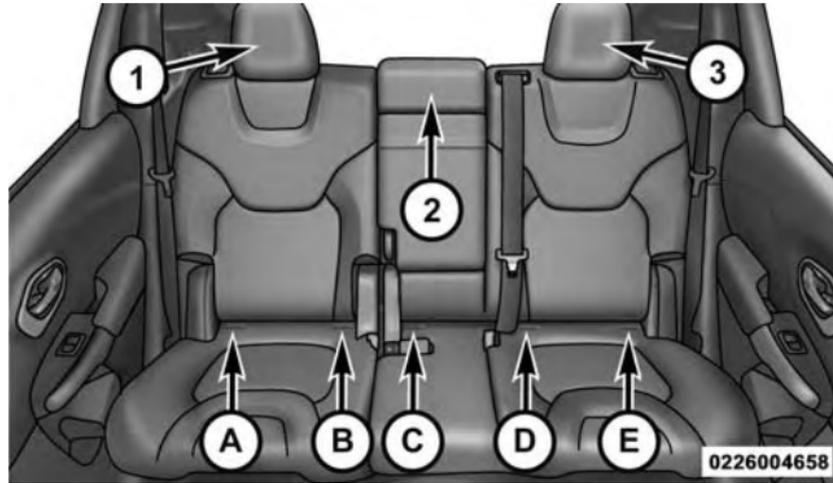
Options for installing two child seats using the LATCH anchorages in this vehicle:
