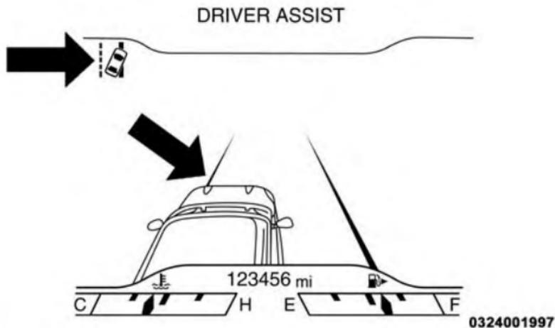
Lane Approached (Flashing White To Gray Thick Line, Solid White Thin Line/Flashing Yellow Indicator)
