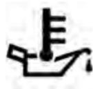
This telltale indicates engine oil temperature is high. If the light illuminates while driving, stop the vehicle and shut off the engine as soon as possible.
