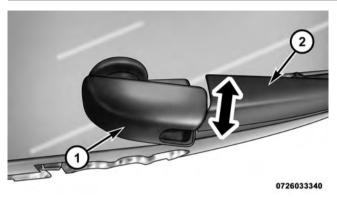
Wiper Pivot Cap In Unlocked Position
