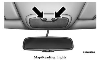
**NOTE:** The lights will remain on until the switch is pushed a second time, so be sure they have been turned off before leaving the vehicle. They will not turn off automatically.
