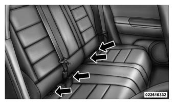
Rear Seat LATCH Anchorages Locating Tether Anchorages
