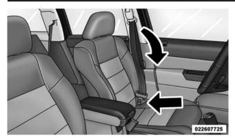
**Inserting Latch Plate Into Buckle**
