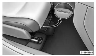
**Right Front Body VIN Location NOTE:** It is illegal to remove or alter the VIN.
