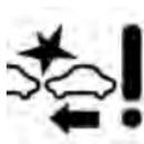
This light warns the driver of a potential collision with the vehicle in front and prompts the driver to take action in order to avoid the collision. For further information, refer to “Adaptive Cruise Control (ACC)” in “Understanding The Features Of Your Vehicle.”
