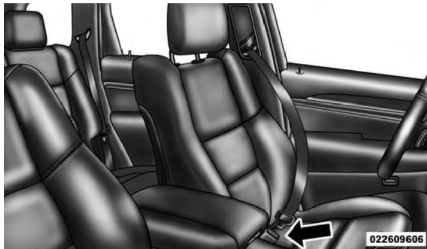
**Inserting Latch Plate Into Buckle**
