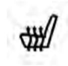
Press the switch once to select HI-level heating. Press the switch a second time to select LO-level heating. Press the switch a third time to shut the heating elements OFF.
