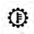
This telltale indicates that the transmission fluid temperature is running hot. This may occur with severe usage, such as trailer towing. If this telltale turns on, safely pull over and stop the vehicle. Then, shift the transmission into NEUTRAL and run the engine at idle or faster until the light turns off.
