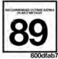
This engine is designed to meet all emissions regulations and provide satisfactory fuel economy and performance when using high-quality unleaded gasoline having an octane range of 87 to 89. Use of 89 octane for optimum performance is recommended. The use of premium gasoline is not recommended, as it will not provide any benefit over plus gasoline in these engines.
