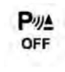
When the ParkSense® switch is pushed to disable the system, the instrument cluster will display the "PARKSENSE OFF" message for approximately five seconds. Refer to "Driver Information Display (DID)" in "Understanding Your Instrument Panel" for further information. When the shift lever/gear selector is moved to REVERSE and the system is disabled, the DID will display the "PARKSENSE OFF" message for as long as the vehicle is in REVERSE.
