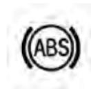
This light monitors the Anti-Lock Brake System (ABS). The light will turn on when the ignition switch is turned to the ON/RUN position and may stay on for as long as four seconds.
