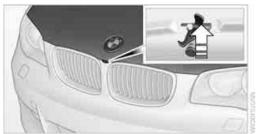
To avoid damage, make sure that the wiper arms are against the windshield before you open the engine compartment. Do not open the engine hood before the engine has cooled down, otherwise injuries may result. ◀ Press the release handle and open the hood.
