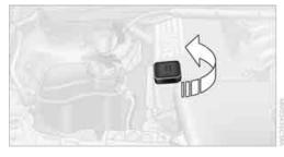
Do not add 1 US guart/1 liter of engine oil until a corresponding message is shown on the Control Display.
