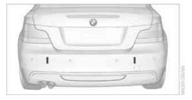
The mounting points are located under the protective covers in the bumper.
