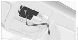
Reattach the lamp cover and reinstall the control unit.
