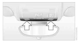
On both sides, use the screwdriver to press on the clip inside the opening.
