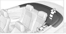
The locking pins must have engaged completely. If they are still visible: close the convertible top box cover as far as necessary until the locking bolts engage audibly, then slowly open the cover. During this process, do not close the convertible top box cover completely.
