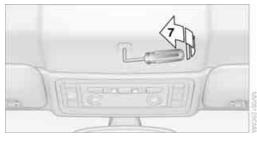
10. Turn the Allen wrench all the way to the left, arrow 7, until the front convertible top frame is locked to the windshield frame. The rear convertible top frame is automatically pressed down onto the convertible top box cover and is sealed tight under tension.
