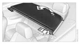
Fold up the top section of the wind deflector, arrow 6.
