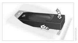
To remove the snap-in adapter: Press area **1**.
