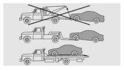
Have your vehicle transported with a tow truck with a so-called lift bar or on a flat bed.
