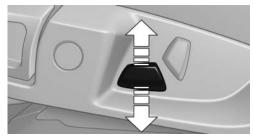
Height: Move the button in the required direction.
