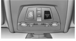
The indicator lamp for the front passenger airbags indicates the operating state of the front passenger airbags.
