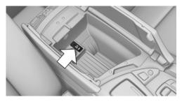
This can be used to connect an external audio device, such as a CD or MP3 player.
