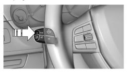
Press the computer button on the turn signal lever.
