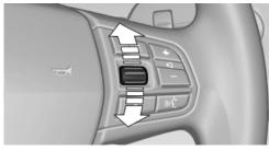
Press a button on the right side of the steering wheel or turn the thumbwheel to activate the required list.
