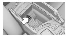
The USB audio interface is in the center armrest. Connect using a flexible adapter cable to protect the USB audio interface and the USB device against physical damage.
