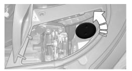
3. Unscrew the bulb holder counterclockwise.
