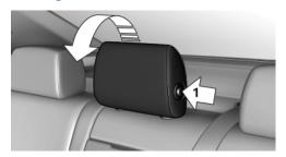
Press the button, arrow 1, and fold the head restraint forward.
