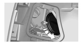
Unscrew the cap, remove it, and change the bulb.
