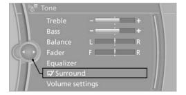
When surround is activated, multi-channel playback is simulated when a stereo audio track is played.
