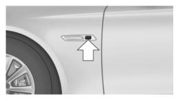
The ultrasounds sensors used to measure parking spaces are located in the side turn signals.
