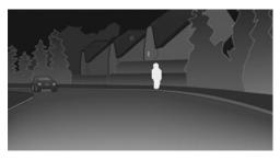
The pedestrian detection and warning system only operates in darkness and only when a heat image is displayed.
