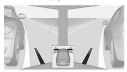
Guidelines at the bottom of the image show the position of the front of the vehicle.
