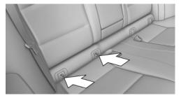
Mounts for the lower LATCH anchors are located behind the indicated covers.
