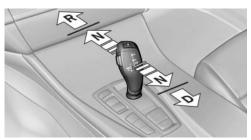
Briefly push the selector lever in the desired direction, beyond a resistance point if necessary.
