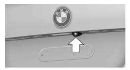
The camera lens is located in the handle of the trunk lid. The image quality may be impaired by dirt.
