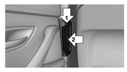
Thumbwheel for opening and closing the vents continuously, arrow 1.
