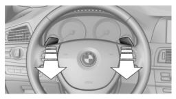
The shift paddles on the steering wheel allow you to shift gears quickly while keeping both hands on the steering wheel.
