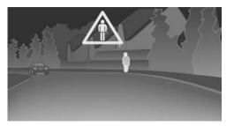
If the system detects a person in the defined area in front of the vehicle and if there is the danger of a collision with this person, a warning symbol appears in the Control Display and Head-up Display\*.
