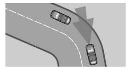
If the desired speed is too high for a curve, the speed is reduced slightly in the curve, although curves cannot be anticipated in advance. Therefore, drive into a curve at an appropriate speed. In tight curves, situations may result due to the restricted detection range of the system in which a vehicle driving shead of you may not be
