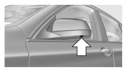
The objectives of the Top View cameras are located at the bottom of the exterior mirror housings. The image quality may be impaired by dirt. Clean the lens, refer to page 276.
