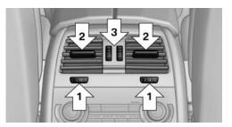
Thumbwheels\* for adjusting the temperature, arrows 1.
