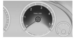
Always avoid engine speeds in the red warning field. In this range, the fuel supply is interrupted to protect the engine.
