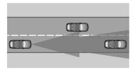
It responds to stationary or moving objects that are within the detection range of the radar system.
