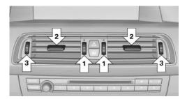
Thumbwheels\* for adjusting the temperature, arrows 1.
