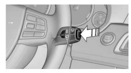
Press the button on the wiper lever.
