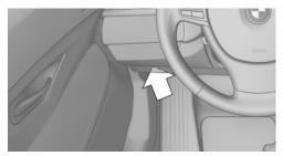
There is an OBD socket on the driver's side for checking the primary components in the vehicle emissions.
