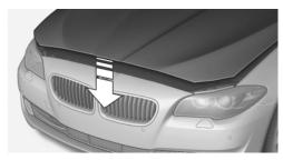
Let the hood drop from a height of approx. 16 in/ 40 cm and push down on it to lock it fully. The hood must audibly engage on both sides.
