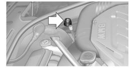
The so-called starting aid terminal in the engine compartment acts as the battery's positive terminal.
