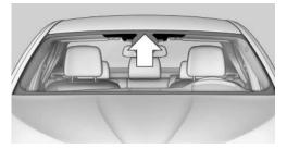
The marked area is not covered with heat reflective coating.
