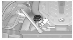
When the indicator lights up in the instrument cluster, add 1 US quart/liter of engine oil within the next 125 miles/200 km.
