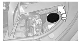
Unscrew the bulb holder counterclockwise.
