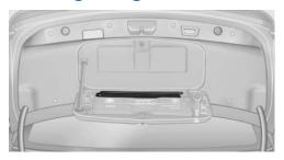
The warning triangle is located in the container on the inside of the trunk lid.
