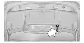
The screw-in tow fitting should always be carried in the vehicle. It can be screwed in at the front or rear of the BMW. It is located in the container on the inside of the trunk lid.
