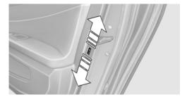
Push the locking lever on the rear doors down. The door can now be opened from the outside only.
