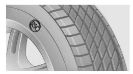
RSC label on the tire sidewall.
