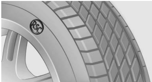
RSC label on the tire sidewall.
