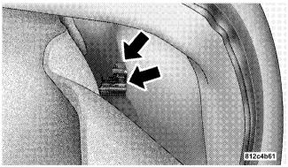
7. Pull the taillamp assembly clear from the vehicle to access the bulbs.
