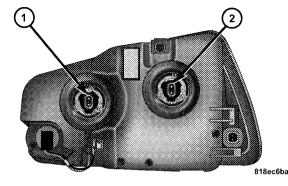
1 — High Beam Headlamp Bulb 2 — Low Beam Headlamp Bulb
