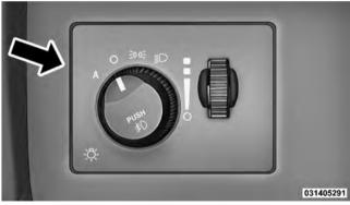
Rotate the headlight switch clockwise to the first detent for parking light and instrument panel light operation. Rotate the headlight switch to the second detent for headlight, parking light and instrument panel light operation.
