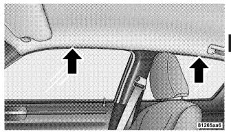
Supplemental Side Airbag Inflatable Curtains (SABIC) NOTE:
