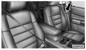
Pulling Out the Lap/Shoulder Belt Latch Plate
