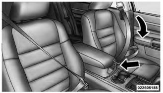
Inserting Latch Plate into Buckle
