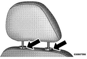
**Removing Head Restraint**
