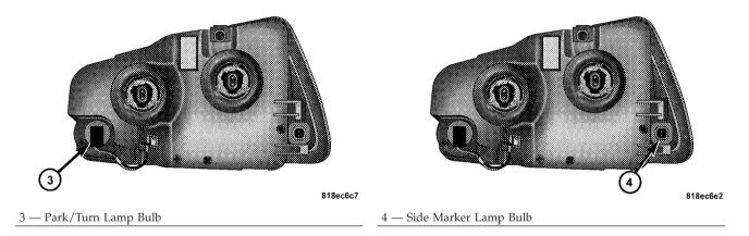
Low Beam Headlamp, High Beam Headlamp, and Park/Turn Lamp — Models with High Intensity Discharge Headlamps (HID)
