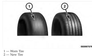
These indicators are molded into the bottom of the tread grooves. They will appear as bands when the tread depth
