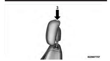
3 — Final Downward Movement To Engage Locking Mechanism
