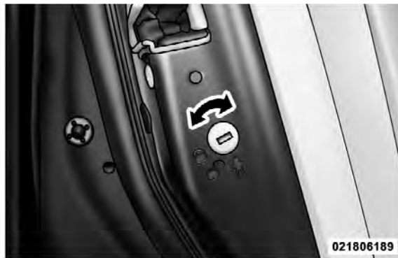
Child-Protection Door Lock Function
