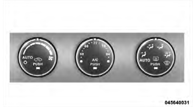
Automatic Temperature Control
