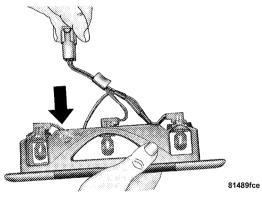
4. Turn desired bulb socket 1/4-turn and remove socket and bulb from housing.
