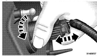
**NOTE:** The headlamp bulb is a halogen bulb. Take care not to touch the bulb with your fingers. Body oils from your fingers could cause excessive heat buildup which reduces bulb life.
