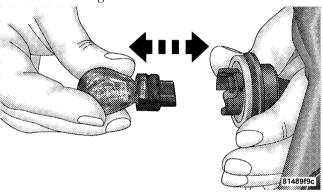
5. Reverse this procedure to install bulb and housing. Place the two raised blocks past the body.
