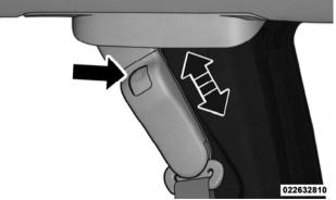
Adjustable Upper Shoulder Belt Anchorage (Extended Cab)
