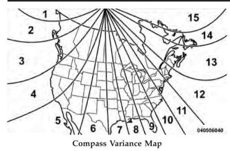
To set the variance: Turn the ignition ON and set the display to "Compass/Temperature." Press and hold the RESET button approximately five seconds. The last variance zone number will be displayed. Press the STEP
