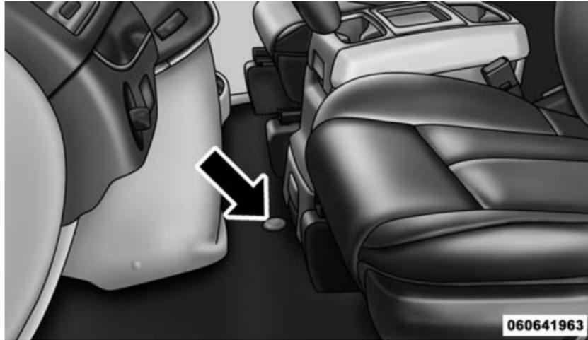
Winch Cover Assembly Plug (If Equipped)
