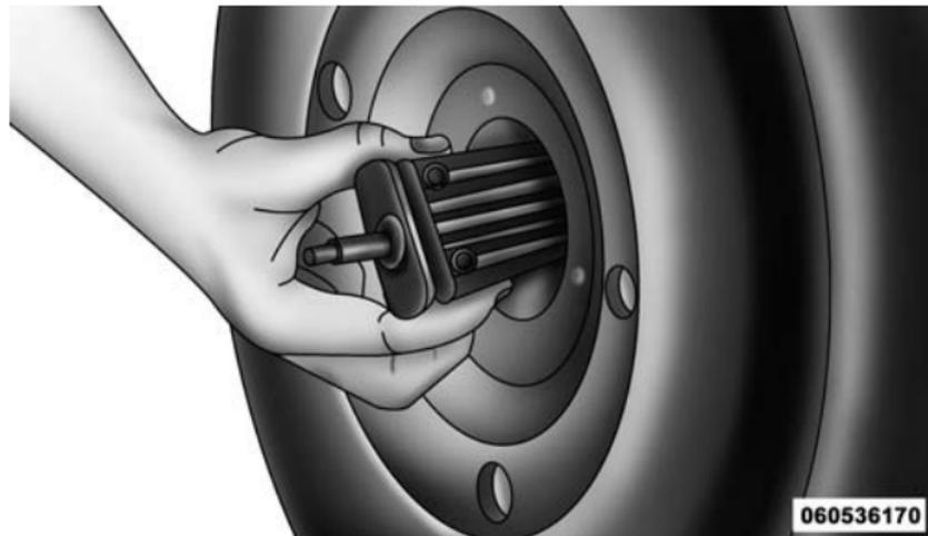
Removing Wheel Spacer
