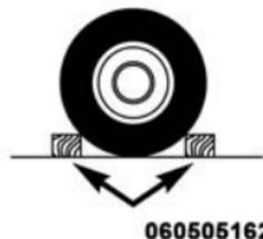
6. Block both the front and rear of the wheel diagonally opposite the jacking position. For example, if changing the right front tire, block the left rear wheel.
