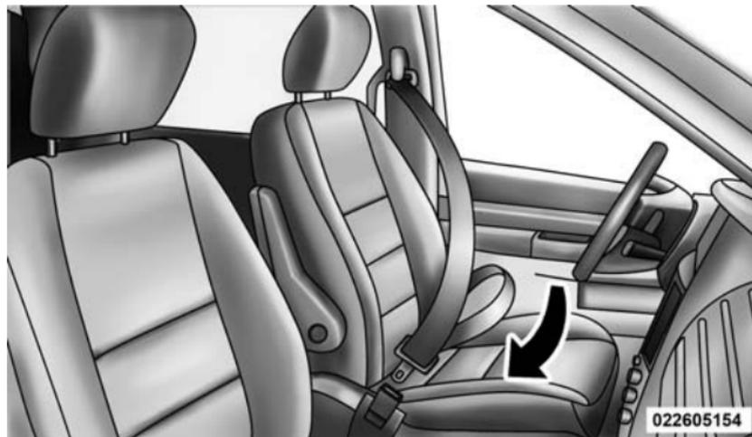
Inserting Latch Plate Into Buckle
