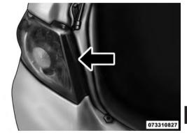
Tail Lamp Housing4. Twist and remove socket from lamp.
