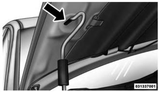
Hood Prop Rod Hole Location Before closing the hood, make sure to stow the prop rod in its proper location.
