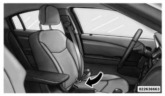
**Inserting Latch Plate Into Buckle**
