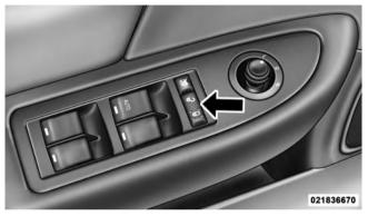
Power Door Lock Switch Automatic Door Locks — If Equipped
