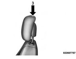
3 — Final Downward Movement To Engage Locking Mechanism
