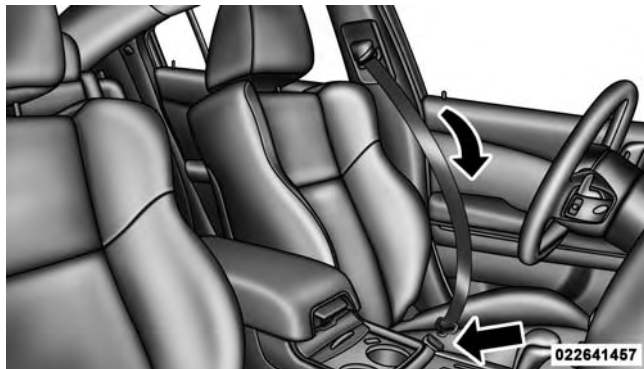
Pulling Out The Lap/Shoulder Belt Latch Plate
