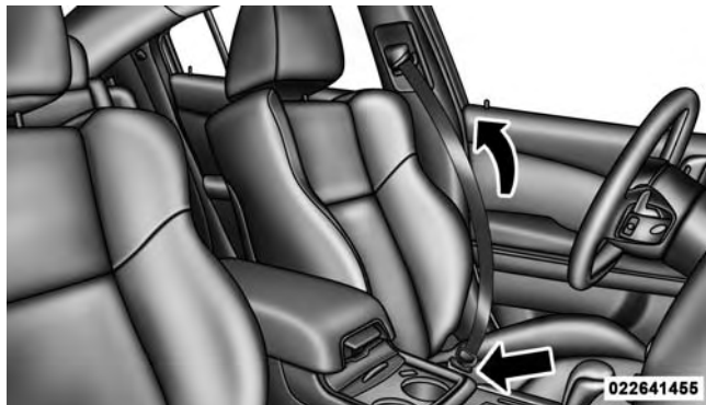
Removing Slack From Belt
