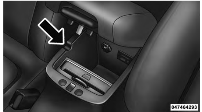
Center Console USB/AUX Connector Port Cable Routing
