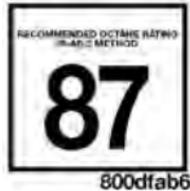
This engine is designed to meet all emissions regulations and provide excellent fuel economy and performance when using high-quality unleaded “regular” gasoline having an octane rating of 87. The use of premium gasoline is not recommended, as it will not provide any benefit over regular gasoline in these engines.
