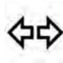
The arrow will flash with the exterior turn signal when the turn signal lever is operated.
