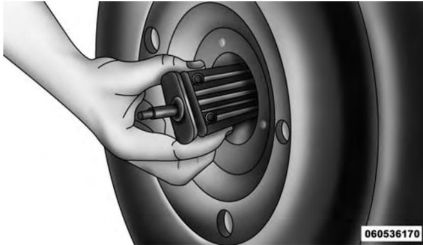
Removing Wheel Spacer
