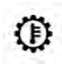
This light indicates that the transmission fluid temperature is running hot. This may occur with severe usage, such as trailer towing. If this light turns on, safely pull over and stop the vehicle. Then, shift the transmission into NEUTRAL and run the engine at idle or faster until the light turns off.
