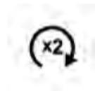
Press and release the REMOTE START button on the RKE transmitter twice within five seconds. The vehicle doors will lock, the parking lights will flash and horn will chirp twice (if programmed). Then, the engine will start and the vehicle will remain in the Remote Start mode for a 15-minute cycle.
