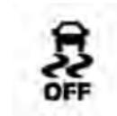
The "ESC Off" switch is located in the center switch bank, next to the hazard flasher switch.
