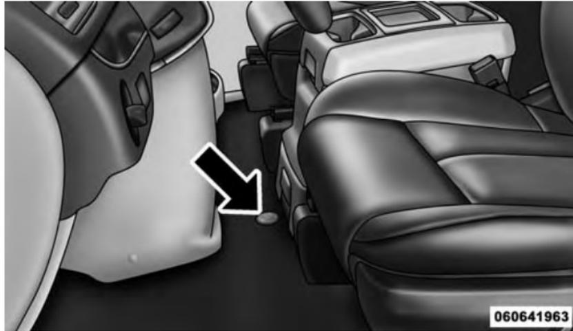
Winch Cover Assembly Plug (If Equipped)
