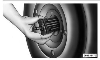
Removing Wheel Spacer
