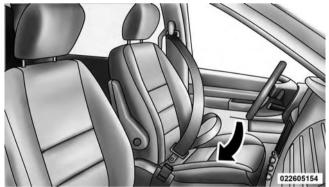
**Inserting Latch Plate Into Buckle**
