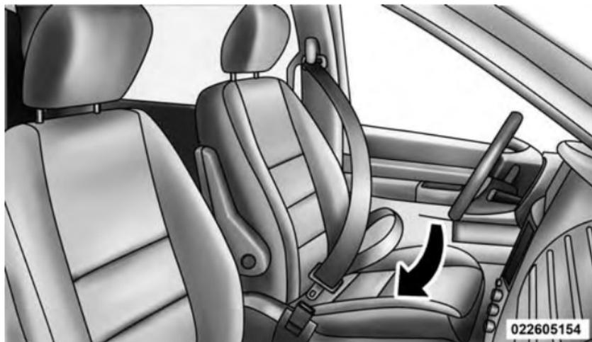
Inserting Latch Plate Into Buckle
