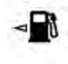
The arrow in this symbol is a reminder that the Fuel Filler Door is located on the left side of the vehicle.
