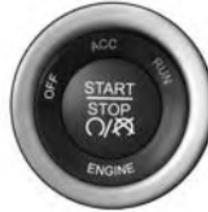
This feature allows the driver to operate the ignition switch with the push of a button, as long as the Remote Start/Keyless Enter-N-Go™ Key Fob is in the passenger compartment.
