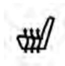
Touch the “Driver” or “Pass” seat soft-key (located on the Uconnect® display) once to select HI-level heating. Touch the soft-key a second time to select LO-level heating. Touch the soft-key a third time to shut the heating elements OFF.
