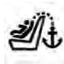
In addition, there are tether strap anchors located behind each rear seatback, near to the floor.
