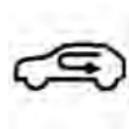
When outside air contains smoke, odors, or high humidity, or if rapid cooling is desired, you may wish to recirculate interior air by
