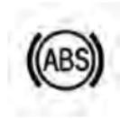
The Anti-Lock Brake Light monitors the ABS. The light will turn on when the ignition switch is turned to the ON position and may stay on for as long as four seconds.
