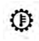
This light indicates that the transmission fluid temperature is running hot. This may occur with severe usage, such as trailer towing. If this light turns on, safely pull over and stop the vehicle. Then, shift the transmission into NEUTRAL and run the engine at idle or faster until the light turns off.
