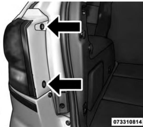
**Inboard Tail Lamp Housing Fasteners**
