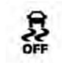
The “ESC OFF Indicator Light” indicates the Electronic Stability Control (ESC) is partially off.
