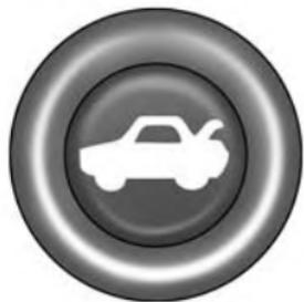
The trunk lid can be released from inside the vehicle by pushing the TRUNK RELEASE button located on the instrument panel to the left of the steering wheel.
