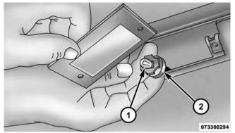
5. Reattach the lamp to the rear fascia, and then install the screws.
