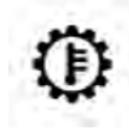
This telltale indicates that the transmission fluid temperature is running hot. This may occur with severe usage, such as trailer towing.
