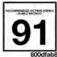
This engine is designed to meet all emission regulations and provide satisfactory fuel economy and performance when using high-quality unleaded "regular" gasoline having an octane rating of 87. For optimum performance and fuel economy the use of 91 octane or higher is recommended.
