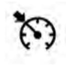
This light will turn on when the electronic speed control is SET. For further information, refer to “Electronic Speed Control” in “Understanding The Features Of Your Vehicle.”
