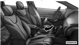
**Inserting Latch Plate Into Buckle**
