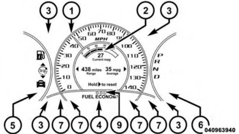
1 — Speedometer (Digital or Analog) (km/h or mph)
