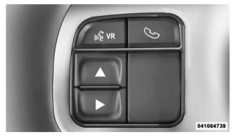
EVIC Steering Wheel Buttons (Two-Button EVIC Controls)
