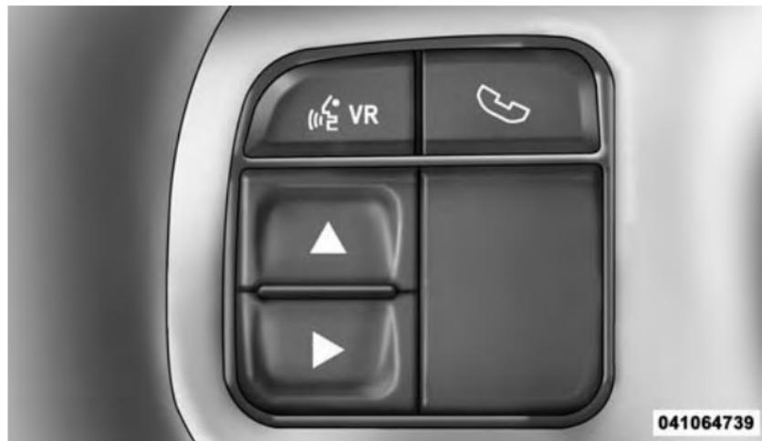
EVIC Steering Wheel Buttons (Two-Button EVIC Controls)
