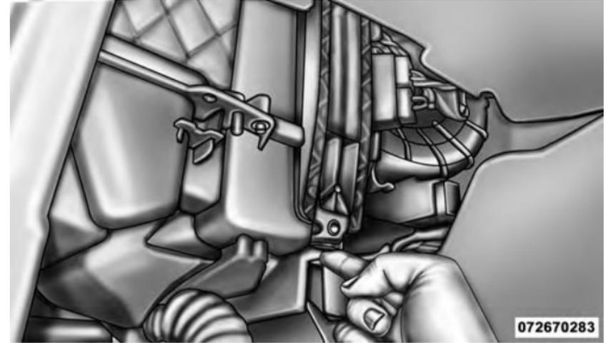
Filter Cover Retaining Tab
