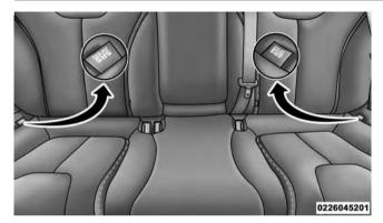
Rear Supplemental Seat-Mounted Side Air Bag Label The SABs may help to reduce the risk of occupant injury during certain side impacts, in addition to the injury reduction potential provided by the seat belts and body structure.
