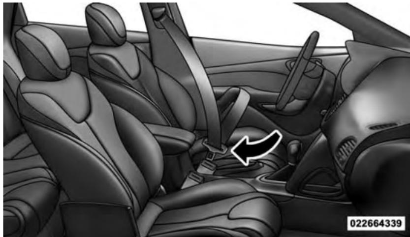
**Inserting Latch Plate Into Buckle**
