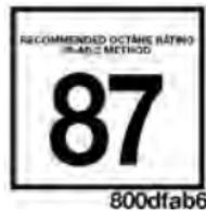
This engine is designed to meet all emissions regulations and provide excellent fuel economy and performance when using high-quality unleaded "regular" gasoline having an octane rating of 87.
