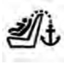
There are tether strap anchorages behind each rear seating position located in the panel between the rear seatback and the rear window. They are found under a plastic cover with the tether anchorage symbol on it.
