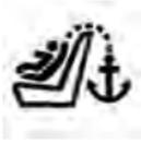
1. Look behind the seating position where you plan to install the child restraint to find the tether anchorage. You may need to move the seat forward to provide better access to the tether anchorage. If there is no top tether anchorage for that seating position, move the child restraint to another position in the vehicle if one is available.
