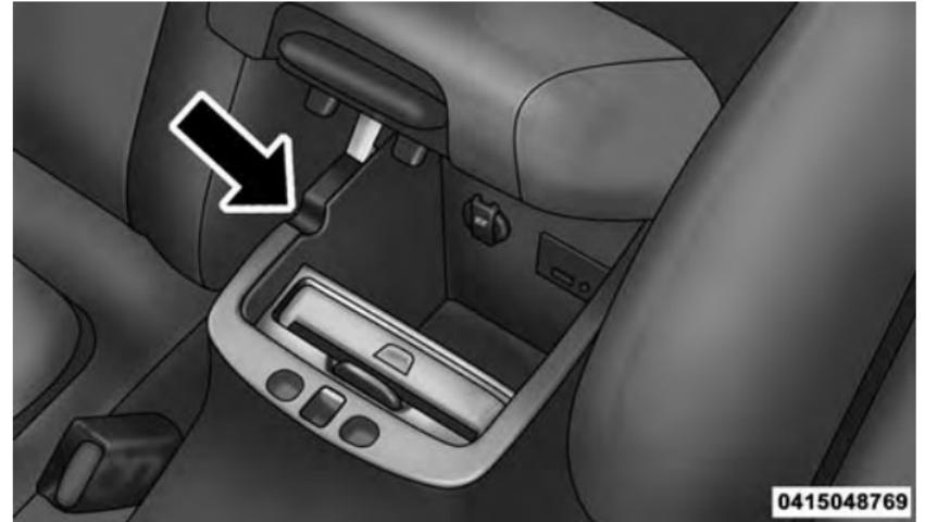
Center Console USB/AUX Connector Port Cable Routing
