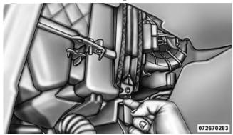
Filter Cover Retaining Tab
