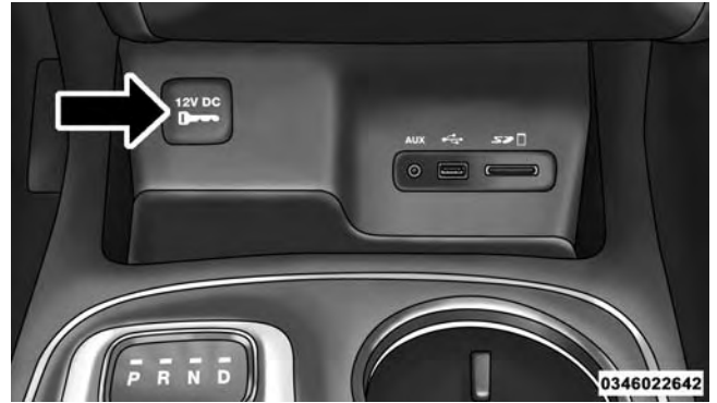
Front Power Outlet
