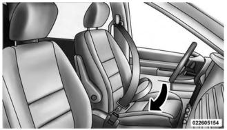
Inserting Latch Plate Into Buckle
