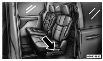
Seatback Recliner Lever, Seat Tumble, And Head Restraint Fold Lever
