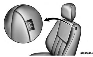
Front Supplemental Seat-Mounted Side Air Bag Label The SABs may help to reduce the risk of occupant injury during certain side impact and certain rollover events, in addition to the injury reduction potential provided by the seat belts and body structure.
