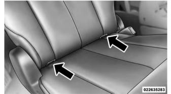
LATCH Anchorages (Second Row Anchorages Shown)
