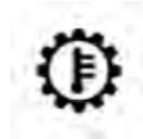
This light indicates that the transmission fluid temperature is running hot. This may occur with severe usage, such as trailer towing. If this light turns on, safely pull over and stop the vehicle. Then, shift the transmission into NEUTRAL and run the engine at idle or faster until the light turns off.
