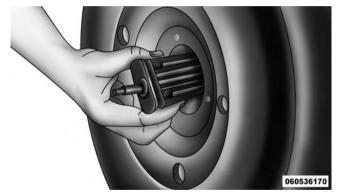
Removing Wheel Spacer
