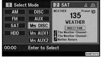
Select VES $^{\text{TM}}$  DISC Mode On The VES $^{\text{TM}}$  Screen
