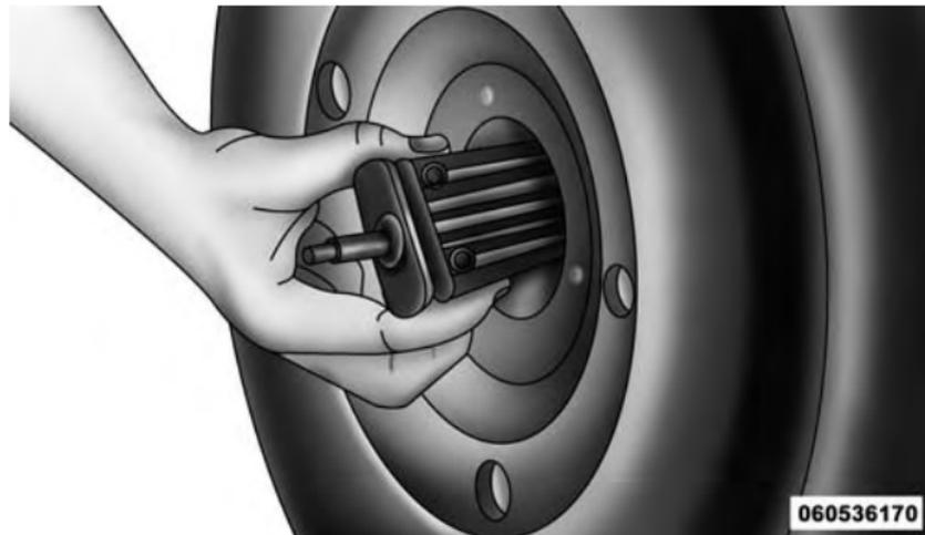
Removing Wheel Spacer
