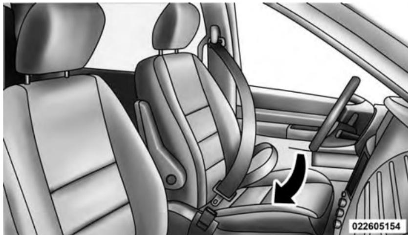
**Inserting Latch Plate Into Buckle**
