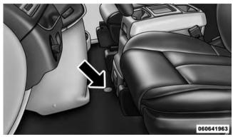
Winch Cover Assembly Plug (If Equipped)
