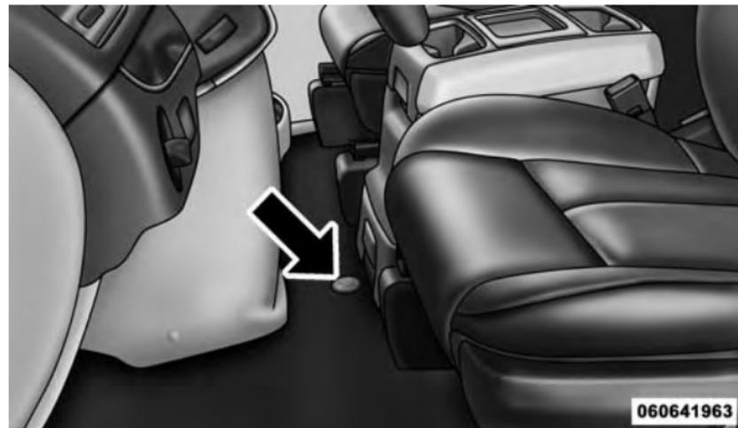
Winch Cover Assembly Plug (If Equipped)
