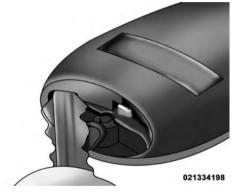
**Inserting Key Into Transmitter Case Slot**
