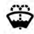
This light will turn on to indicate the windshield washer fluid is low.
