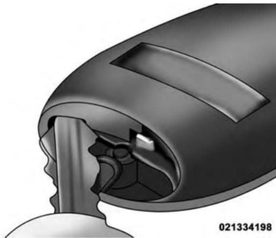
Inserting Key Into Transmitter Case Slot
