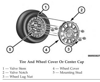
3. Align the valve notch in the wheel cover with the valve stem on the wheel. Install the cover by hand,
