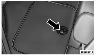
In-Floor Storage The liner can be removed for easy cleaning.
