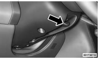
Tilt/Telescoping Steering Control Handle
