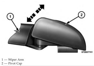
**NOTE:** The rear wiper arm cannot be raised fully upward unless the pivot cap is raised first.
