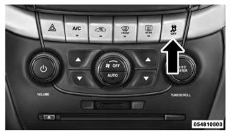
**NOTE:** To improve the vehicle's traction when driving with snow chains, or when starting off in deep snow, sand, or gravel, it may be desirable to switch to the "Partial Off" mode by momentarily pressing the "ESC OFF" button. Once the situation requiring "Partial Off" mode is overcome, turn ESC back on by momentarily pressing the "ESC OFF" button. This may be done while the vehicle is in motion.
