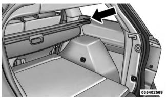
Installing Retractable Cargo Area Cover
