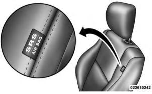
**Front Supplemental Seat-Mounted Side Air Bag Label** The SABs may help to reduce the risk of occupant injury during certain side impact and certain rollover events, in addition to the injury reduction potential provided by the seat belts and body structure.
