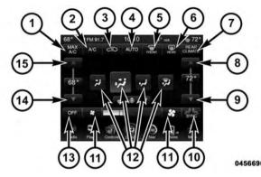
Uconnect® 8.4 Automatic 3 — Zone Temperature Controls — Buttons On The Touchscreen Button Descriptions (Applies To Both Buttons On The Faceplate And Buttons On The Touchscreen)
