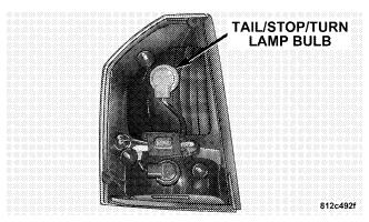
8. Pull the appropriate bulb to remove it from the socket.
