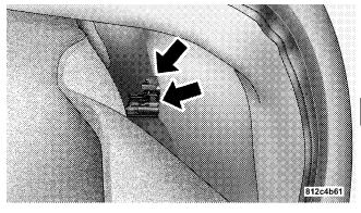
7. Pull tail light assembly clear from vehicle to access bulbs. Turn bulb sockets counter-clockwise to remove.
