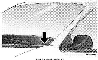
VIN LOCATION NOTE: It is illegal to remove the VIN plate.
