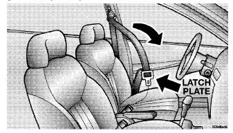
Latch Plate To Buckle 3. When the belt is long enough to fit, insert the latch plate into the buckle until you hear a "click."
