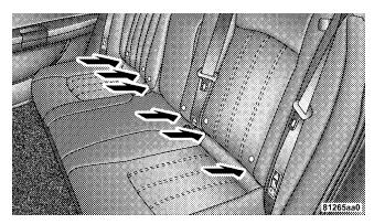
LATCH Anchorages Installing the LATCH-Compatible Child Restraint System
