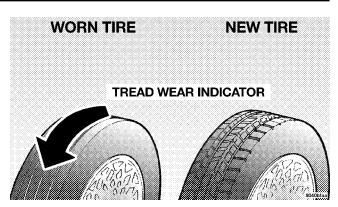
These indicators are molded into the bottom of the tread grooves and will appear as bands when the tread depth becomes 1/16 inch (2 mm). When the tread is worn to the tread wear indicators, the tire should be replaced.
