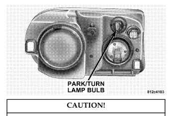
Do not touch the new bulb with your fingers. Oil contamination will severely shorten bulb life. If the bulb comes in contact with an oily surface, clean the bulb with rubbing alcohol.
