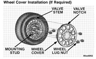
1. Tighten the two lug nuts on the mounting studs on each side of the stud which is in alignment with the valve stem.
