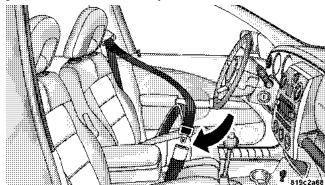
Inserting Latch Plate Into Buckle
