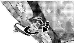
**Engaging Convertible Top Latches** 5. Raise the latch handle into the stowed position.
