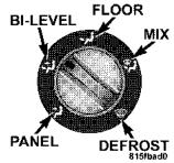
The mode control allows you to choose from several patterns of air distribution. You can select either a primary mode, as identified by the symbols, or a blend of two of these modes. The closer the control is to a particular mode, the more air distribution you receive from that mode.
