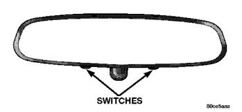
**NOTE:** The lights will remain on until the switch is pressed a second time, so be sure they have been turned off before leaving the vehicle. They will not turn off automatically.
