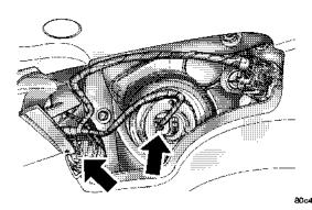
3. Rotate the socket to the left one quarter turn and 7 replace the bulb.
