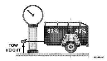
Consider the following items when computing the weight on the rear axle of the vehicle:
