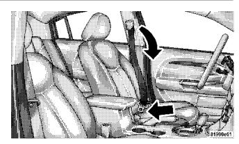
Inserting Latch Plate Into Buckle
