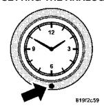
To set the analog clock at the top center of the instrument panel, press and hold the button until the setting is correct. The clock will adjust slowly at first and then quicker the longer the button is held.
