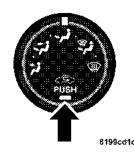
Use this button to choose between outside air intake or recirculation of the air inside the vehicle. A lamp will illuminate when you are in recirculate mode. Only use the recirculate mode to temporarily block out any outside odors, smoke, or dust and to cool the interior rapidly upon initial start up in very hot or humid weather.
