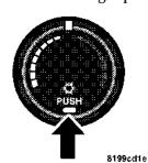
Use this button to engage the Air Conditioning. A lamp will illuminate when the Air Conditioning System is engaged
