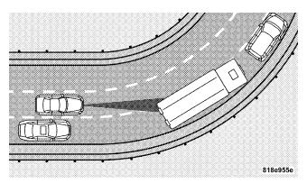
ACC may occasionally provide braking and/or a driver alert that you consider unnecessary. This may be the system's response to signs, guardrails, and other stationary objects in a curve. This may also occur at the base of dramatic hills. This is normal operation and your vehicle does not require service.
