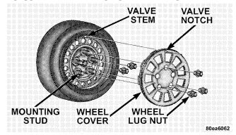
2. Install two lug nuts on the mounting studs, which are on each side of the stud that is in alignment with the valve stem. Install the lug nuts with the cone shaped end of the nut toward the wheel. Lightly tighten the lug nuts. To avoid the risk of forcing the vehicle off the jack, do not tighten the lug nuts fully until the vehicle is lowered to the ground.
