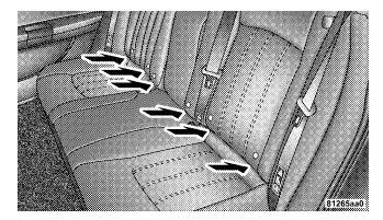
**LATCH Anchorages** Installing the LATCH-Compatible Child Restraint **System**
