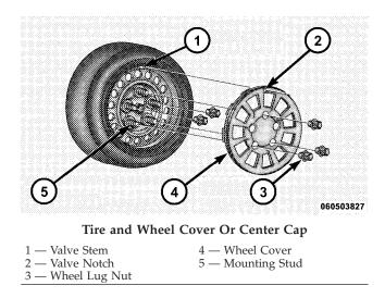
3. Align the valve notch in the wheel cover with the valve stem on the wheel. Install the cover by hand, snapping the cover over the two lug nuts. Do not use a hammer or excessive force to install the cover.
