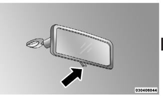
Adjusting Rearview Mirror Automatic Dimming Inside Mirror — If Equipped This mirror automatically adjusts for headlight glare from vehicles behind you. You can turn the feature on or off by pressing the button at the base of the mirror. A light next to the button will illuminate to indicate when the dimming feature is activated.
