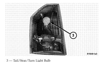
9. Disconnect the bulb from the socket assembly and install the replacement bulb.
