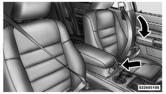
Inserting Latch Plate into Buckle
