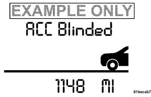
**NOTE:** If the ACC Blinded Warning is active Normal (Fixed Speed) Cruise Control is still available. For additional information refer to "Normal (Fixed Speed) Cruise Control Mode" in this section.
