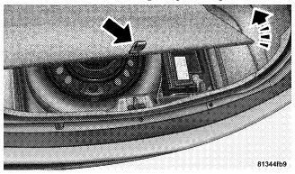
**Opening The Access Panel** 3. Remove the fastener securing the spare tire.
