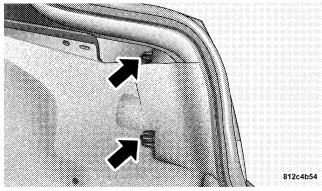
4. Remove the remaining fastener from the back of the tail light assembly.
