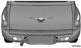
2. Fully compress the clip to get the lamp to come out completely.
