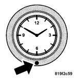
To set the analog clock, located at the top center of the instrument panel, press and hold the button in until the setting is correct. The clock will adjust slowly at first and then quicker the longer the button is held.
