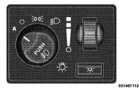
Headlight Switch With Halo Control Assembly
