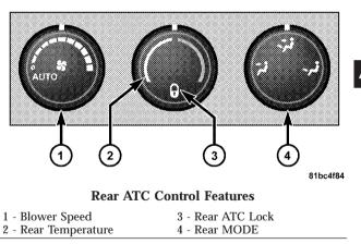
1. Press the REAR LOCK button on the front lower ATC panel. This turns off the REAR LOCK icon in the rear temperature knob.
