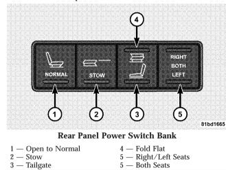
**NOTE:** The third row power seat system includes obstacle detection for safe operation. When the system detects an obstacle, the motors will stop and reverse the motion a short distance to move the seat away from the obstacle. Should this occur, remove the obstacle and press the button again, for the desired position.
