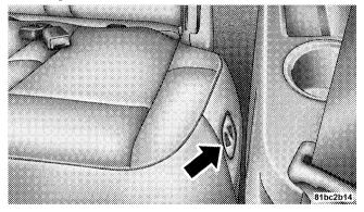
Third Row Power Seat Switch Third Row Power Seat Switch — If Equipped A one-touch power folding seat switch is located in the left rear trim panel as part of a switch bank. The switch is only functional when the liftgate is open and the vehicle is in PARK.
