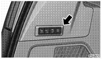
**One Touch Folding Seat Third Row** The rear switch bank allows multiple power folding and unfolding positions for the third row seats.
