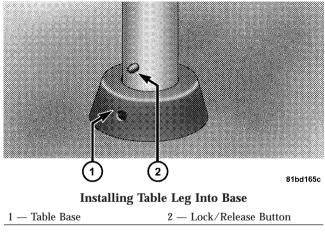
5. Twist the pole in a clockwise rotation until it stops.
