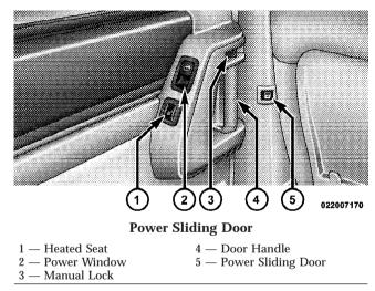
If the inside or outside door handles are used while the power sliding side door is activated, the power sliding door feature will be canceled.
