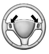
Remote Sound System Controls (Back View Of Steering Wheel)
