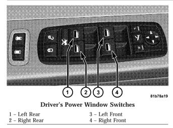
**NOTE:** Power Window switches will also remain active for up to 10 minutes after the ignition switch has been turned to LOCK, depending upon the accessory delay setting. Opening a front door will cancel this feature.
