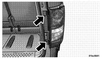
Tail Lamp Housing Fastener Removal
