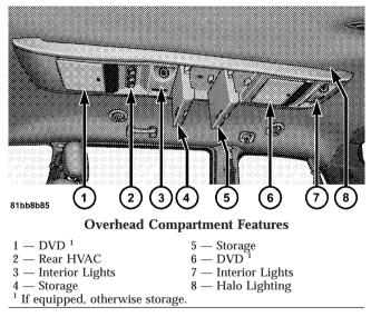
**Rear Courtesy/Reading Lights — If Equipped** The overhead console has two sets of courtesy lights. The lights turn on when a front door, a sliding door or the liftgate is opened. If your vehicle is equipped with Remote Keyless Entry (RKE) the lights will also turn on when the UNLOCK button on the RKE transmitter is pressed.
