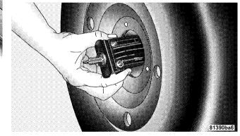
**Squeezing Winch Retainer Tabs**
