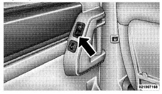
**Sliding Door Power Window Switch** NOTE: The sliding door windows do not fully open, stopping several inches above the window sill.
