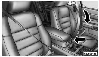
**Inserting Latch Plate into Buckle**
