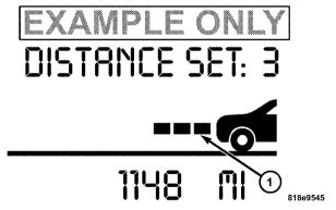
To change the distance setting, push the lever away from you (DISTANCE) and release. Each time this is done, the distance setting adjusts between long, medium, and short.
