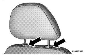
Removing Head Restraint
