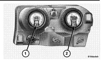
1 — High Beam Headlamp Bulb2 — Low Beam Headlamp Bulb
