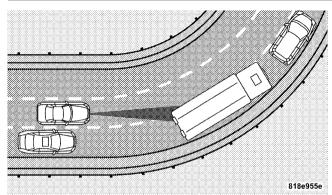
ACC may occasionally provide braking and/or a driver alert that you consider unnecessary. This may be the system's response to signs, guardrails, and other stationary objects in a curve. This may also occur at the base of steep hills. This is normal operation and your vehicle does not require service.
