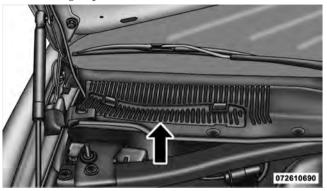
2. Slide the lid on the filter adapter forward and down and remove the used filter.
