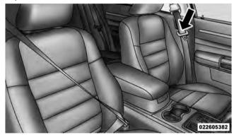
Pulling Out the Lap/Shoulder Belt Latch Plate
