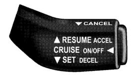
**NOTE:** In order to ensure proper operation, the Electronic Speed Control System has been designed to shut down if multiple Speed Control functions are operated simultaneously. If this occurs, the Electronic Speed Control System can be reactivated by pushing the Electronic Speed Control ON/OFF button and resetting the desired vehicle set speed.
