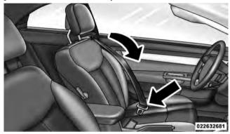
Inserting Latch Plate into Buckle
