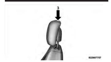
3 — Final Downward Movement To Engage Locking Mechanism
